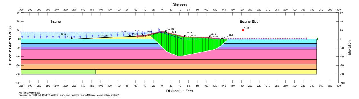
CLASSIFICATION STRATIFICATION SHEAR STRENGTHS AND UNIT WEIGHTS OF THE SOIL WERE BASED ON THE RESULTS OF UNDISTURBED BORINGS. SEE BORING DATA PLATES.
