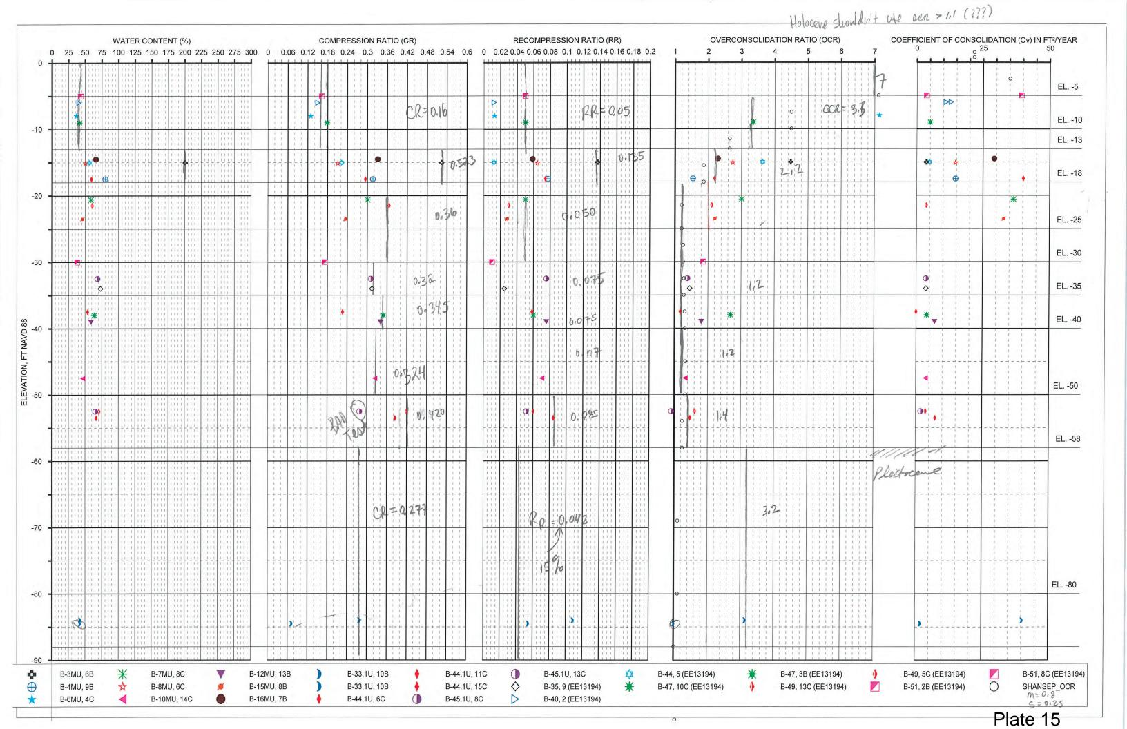
EE 22557 Magnolia Ridge **Consolidation Test Summary**  Homogeneous CL and CH sedimentary clays of low to moderate sensitivity ( $I_p = 20\% - 80\%$ ):  $S = 0.20 + 0.05I_p$ , or simply S = 0.22.  $m = 0.88(1 - C_s/C_c) \pm 0.06$  SD, or simply m = 0.8. Sedimentary deposits of silts and organic soils (Atterberg limits plot below
